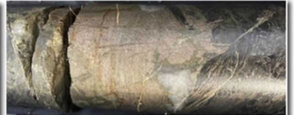
Severn Drillhole ZS140, Typical example (775.7m – 780.4m) of sulphide mineralisation containing tin 10
