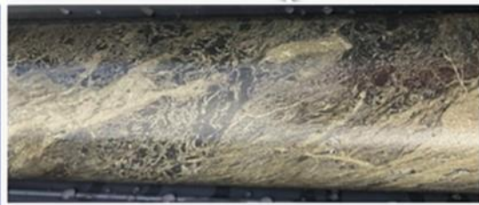
Severn Drillhole ZS140, Typical example (775.7m – 780.4m) of sulphide mineralisation containing tin 10
