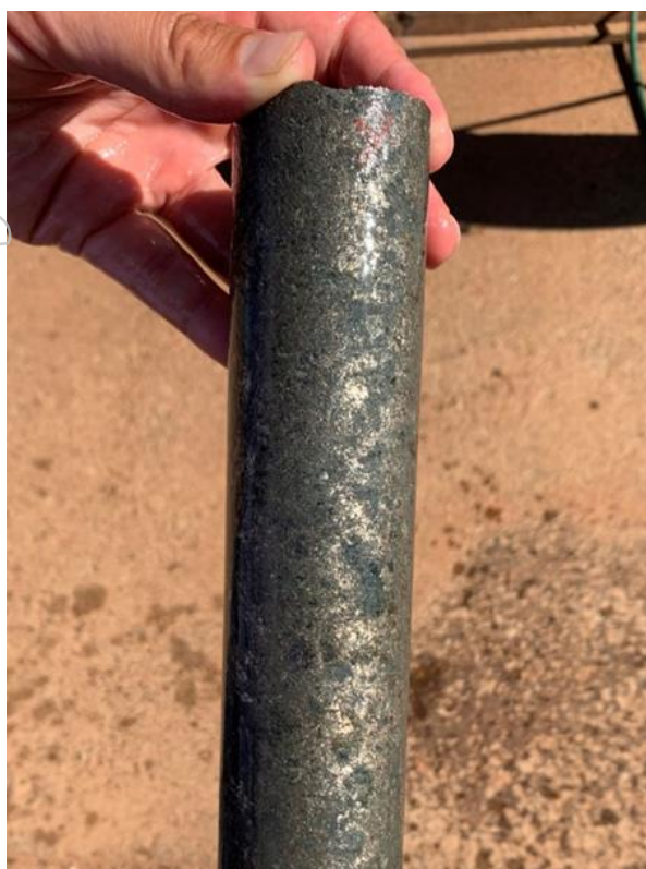
Figure 6: ANDD0005 drill core Massive Ni-Cu sulphides @ 330.0m-330.2m 1.0m @ 3.49% Ni & 0.44% Cu
