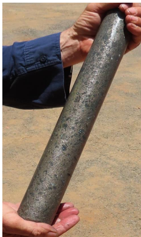
Figure 7: ANDD0006 drill core Massive Ni-Cu sulphides @ 416.9m-417.3m 0.75m @ 3.75% Ni and 0.21% Cu
