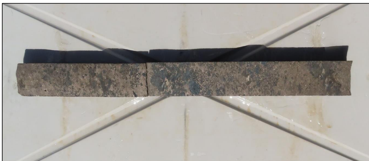
Figure 8: ANDD0011 at VC-23; semi-massive sulphides: 0.67m @ 3.62% Ni & 0.15% Cu
