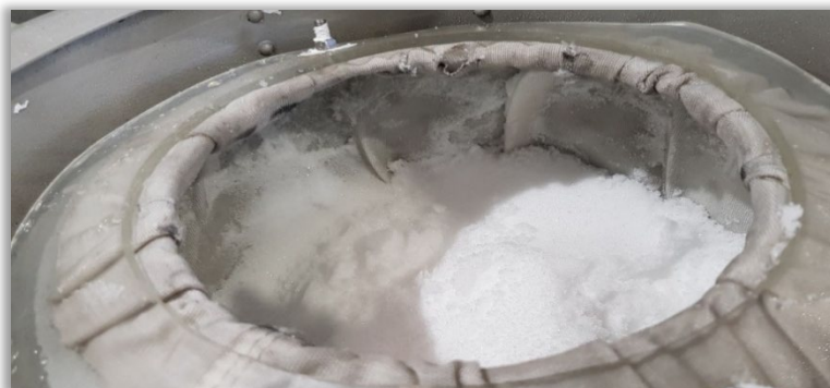
A centrifuge batch of 5N purity aluminium nitrate-nonahydrate product produced at Alpha's demonstration scale facility
