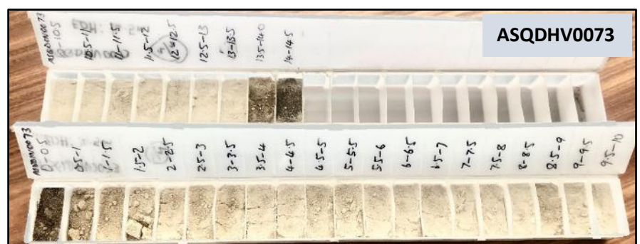
Albany White Hill Project Vacuum drill hole ASQDHFV0073 sample tray showing silica sand intersection from 0.5-13.5 m
