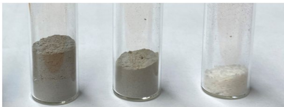
Lithium process residue → Leached residue → Linde type A (4A) zeolite
