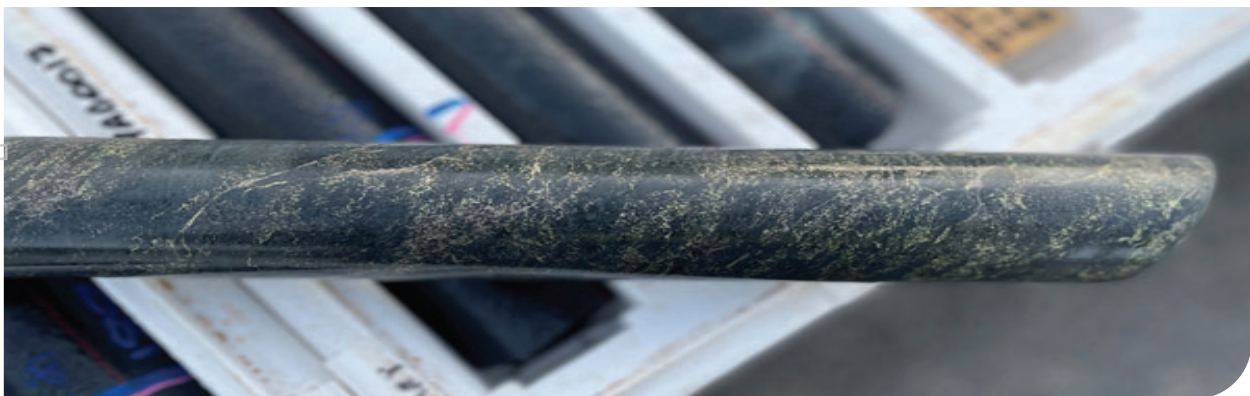
Figure 6. Mineralisation at 308.8m in YAD0017 assaying 4.10g/t PGE (0.77g/t Pd, 3.33g/t Pt), 0.56% Ni & 2.01% Cu.
