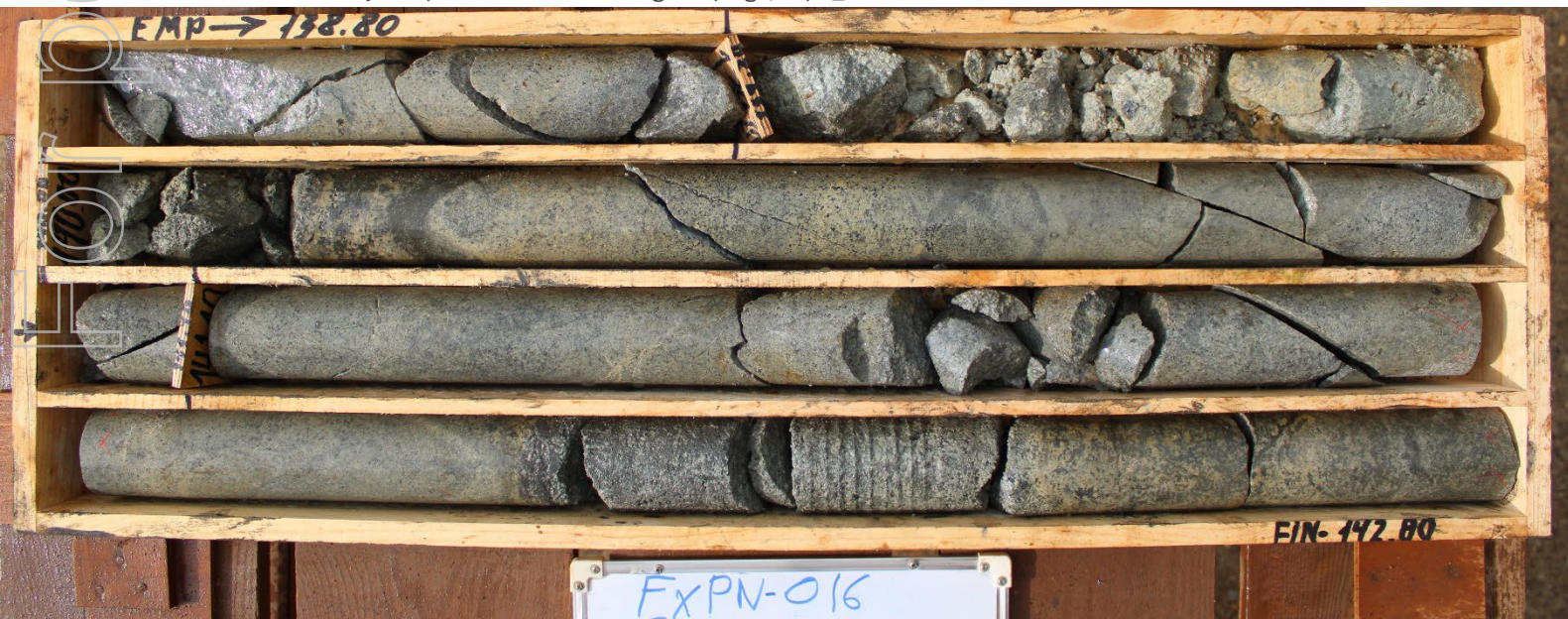
Drill core from recently completed Resource drilling campaign, Expn_016 4m @ 0.69% Sn from 138.8m
