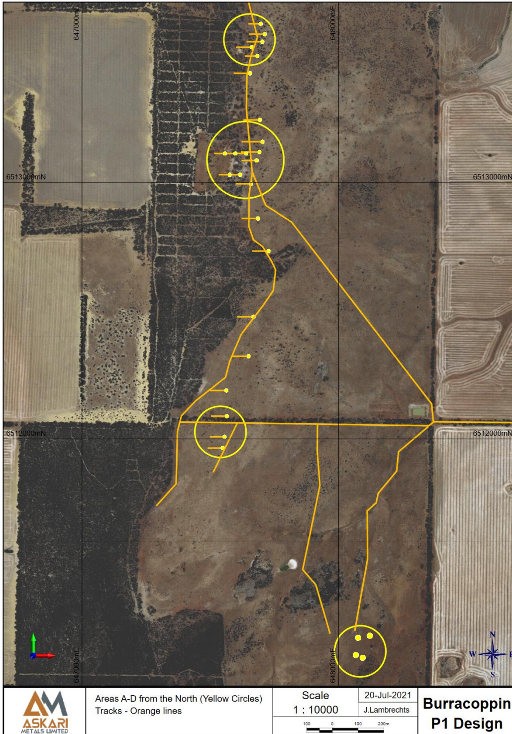
Figure 6: Overview drill design at Burracoppin Gold Project
