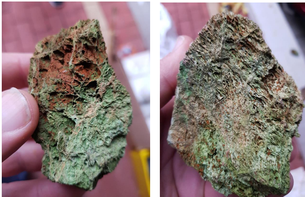
Figure 12 - Visual copper associated with gossan in rock chip samples collected along the Bali Shear Zone.
