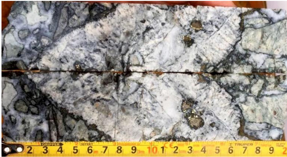
Figure 11: Two halves of cut NQ size core from hole CDH-077 472.1-472.3 metres with abundant visible gold
