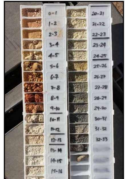
Figure 5: OAR's Gibraltar Project Drill cutting from GBAC069 showing white kaolinitic saprolite developed over gneissic basement material
