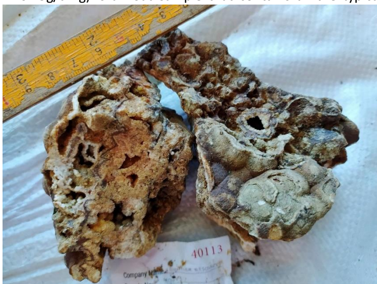
Figure 5: Rock float (SN# 40113) from Kimono Central displaying comb, crustiform, colloform, lattice bladed and botryoidal quartz textures typical of the boiling zone of an epithermal system
