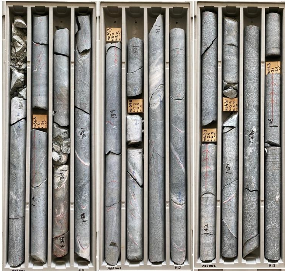
Figure 4: Diamond core from 35 m to 45.5m of Hole MQD0001 in the May Queen gold project
