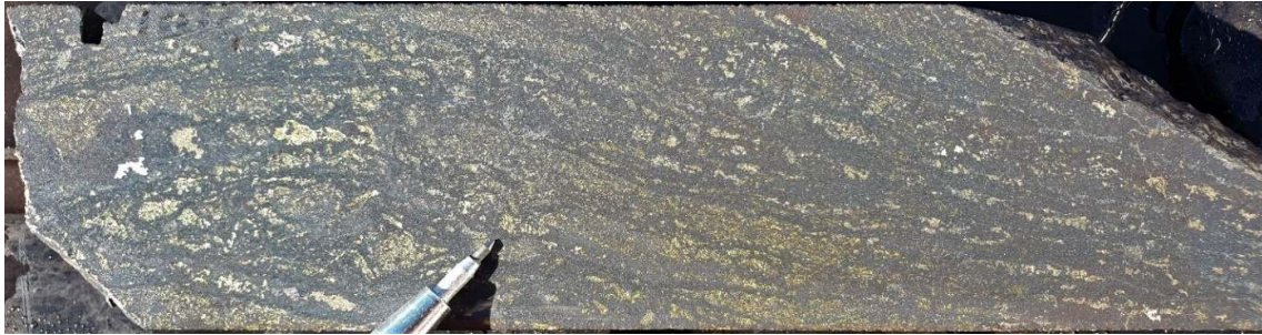
Plate 2c: VUD0019 - 1416.1m. Layered chalcopyrite and lesser pyrite mineralisation in hematite breccia. NQ2 ½ core.
