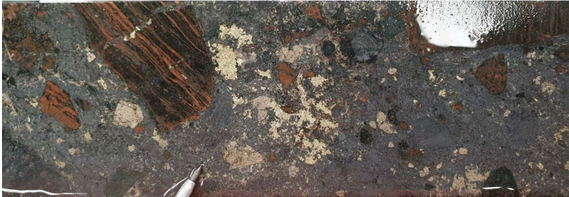
Plate 2d: VUD0019 - 1452.5m. Disseminated and blebby pyrite and lesser chalcopyrite mineralisation in hematite-rich polymictic breccia. NQ2 ½ core.
