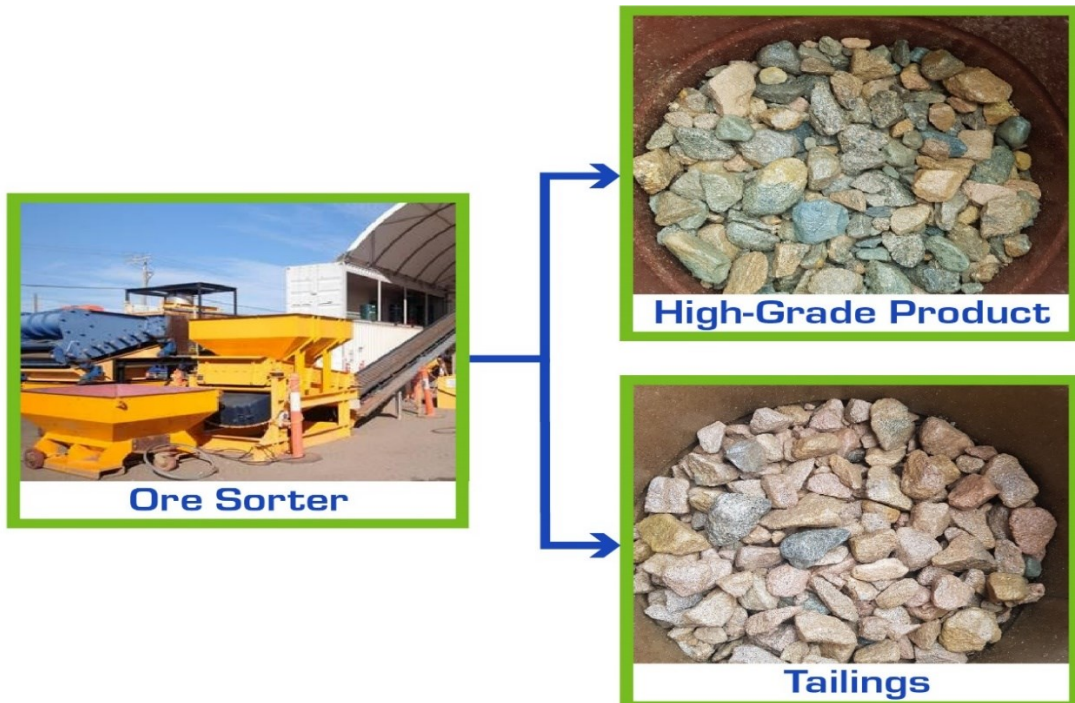
Image 4: ROM feed to the ore sorter before separating into product and tailings
