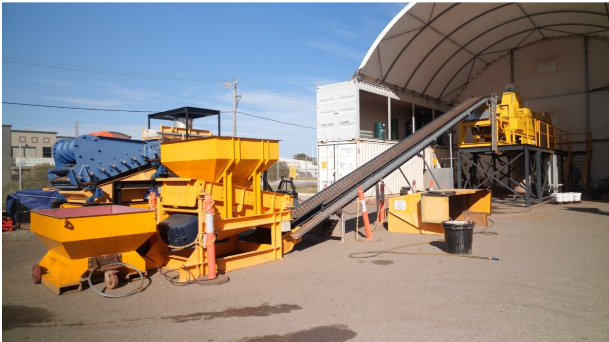
Image 3: Ore sorting facility used during testwork is the same size proposed for use at Kayelekera
