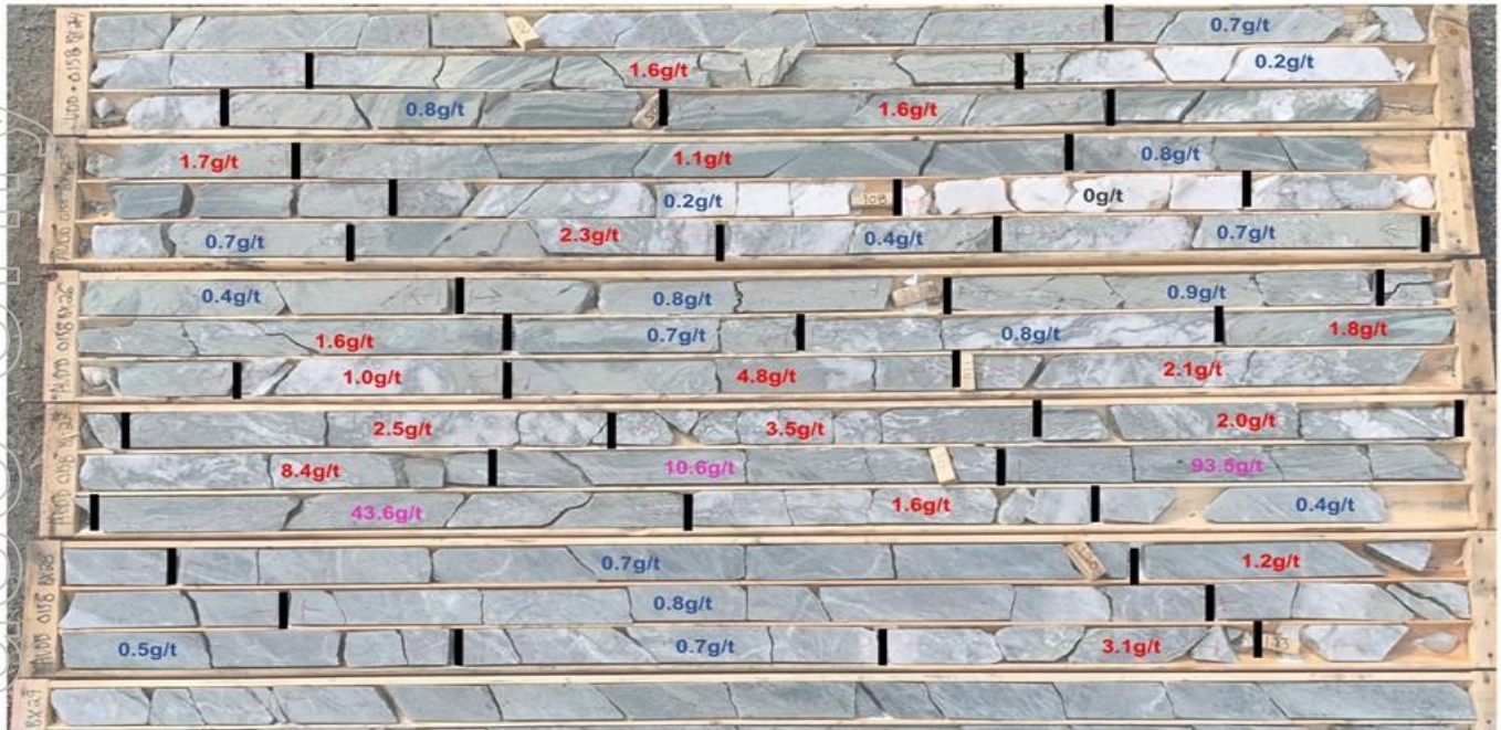
Figure 5: AUDD0158: New Discovery. 102.65m to 123m. Sericite-ankerite-pyrite altered intermediate dyke within sericite-ankerite-pyrite altered Quartz-Feldspar-Porphyry. Alteration to the selvedge of and is related to multiple sheared Quartz-Ankerite-Pyrite veins. Interval is 20.4m @ 5.3g/t Gold including 2.2m @ 39.3g/t Gold from 116m.
