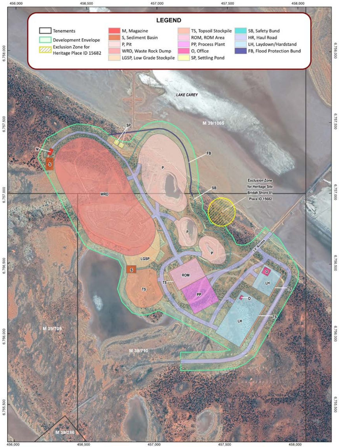
Figure 19: Proposed mine layout for Fortitude Stage 2 mining
