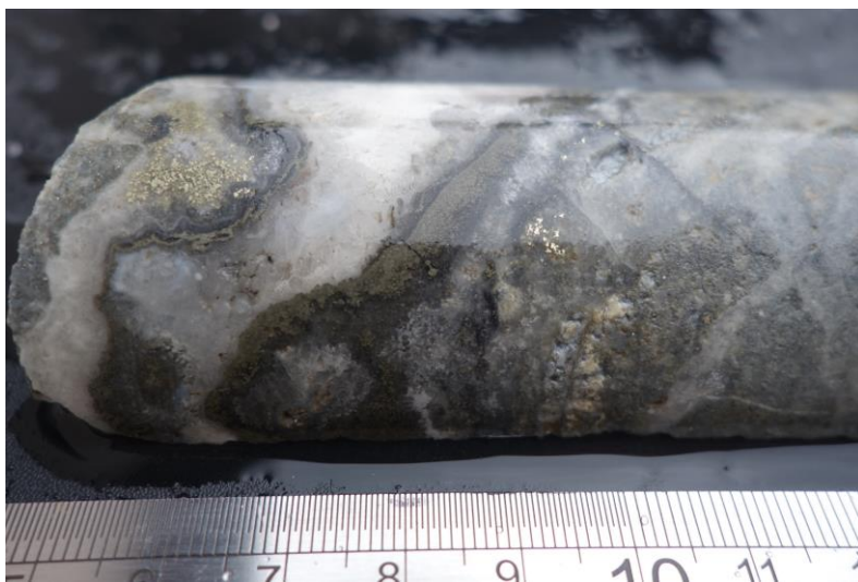
Figure 1: Visible gold in a ~5cm wide, drusy, fine grained, white to grey chalcedonic quartz-pyrite filled vein/stockwork zone at 41.4m in UGA-16
