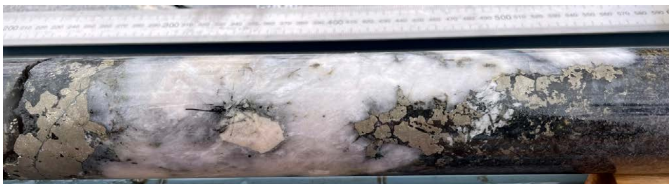
Figure 1: GDRCD007 - 547m, example of a large quartz-calcite vein in altered diorite with semi-massive sulphides pyrite ±Chalcopyrite as well as Chlorite, Actinolite infill.
