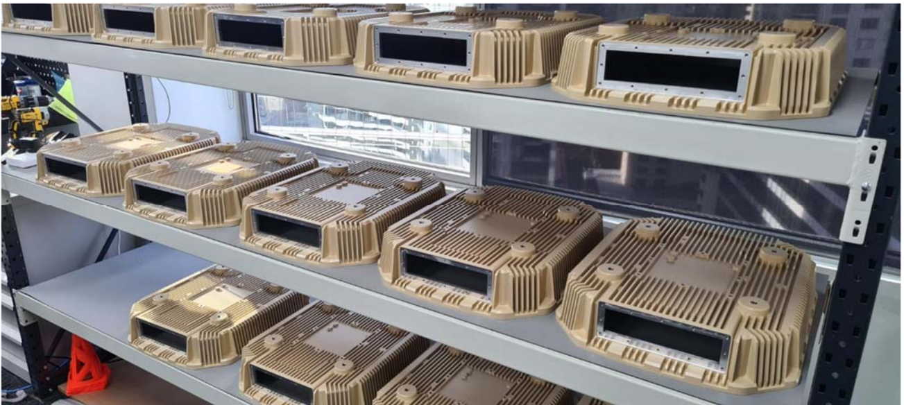
Image: DroneSentry-X™ heatsinks during the manufacturing process
