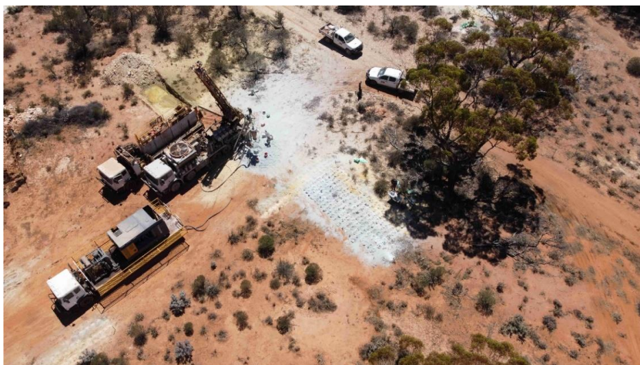
Figure 5. KTE Mining Services RC rig drilling at the Rocky Dam Project.
