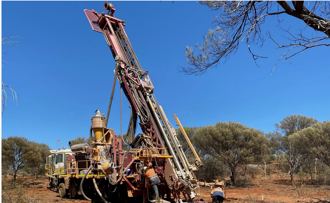
Figure 2: RC drill rig on site at Rover
