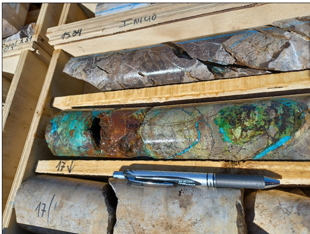
Figure 4: Visual Copper Mineralisation (malachite and chrysocolla) Intersected in Drillhole CMPDD006 at 16m Downhole.
