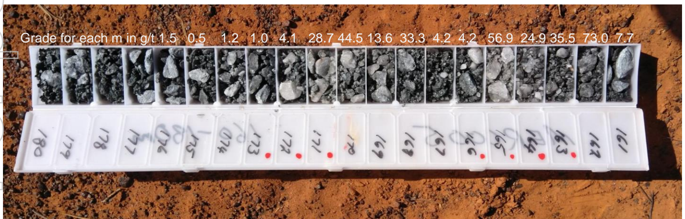
Figure 9: Chip tray from MERC005 with 16m @ 20.92g/t high grade intercept from 161m
