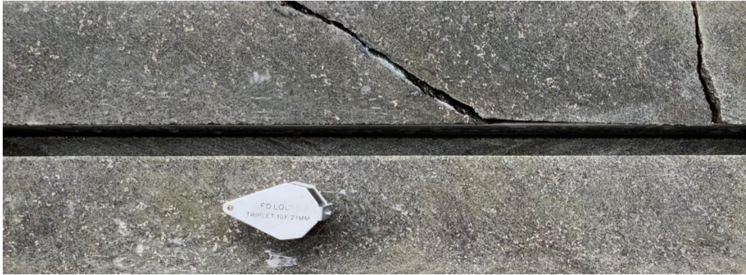
Figure 4 - Disseminated Sulphides over the 148 to 161m interval. The top image has disseminated sulphides throughout. The bottom image is zoomed in to a portion of the core to make them more visible.
