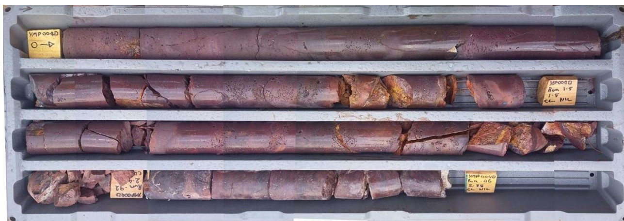
Figure 1. Hematite sandstone with hematite enrichment in drill hole YMP004D from surface to 2.88m depth.
