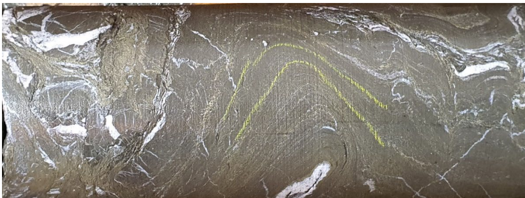
Figure 5. CD21-001 at down-hole depth of 47.5m. Very fine-grained massive pyrite and chalcopyrite with soft sediment folding and slumping. This interval assayed 9.3% Cu and 15.2g/t Ag. Scale bar approx. 5cm.
