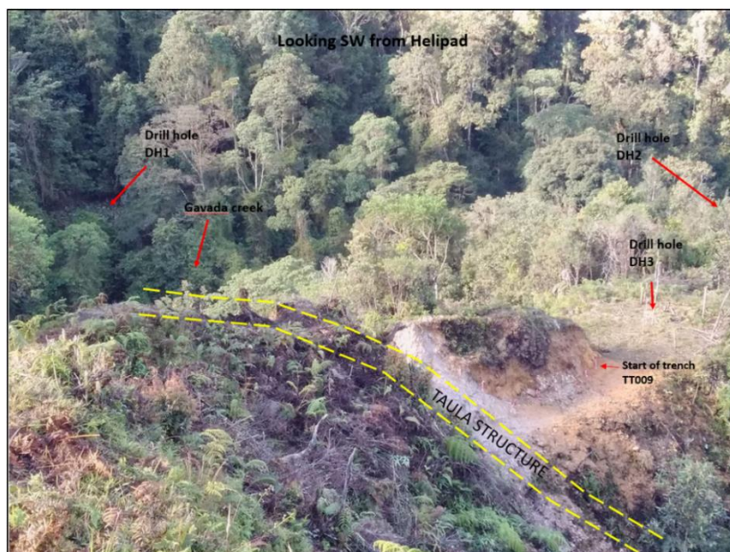
Figure 24: Taula Structure at Trench TT009 with 8m @ 2.83g/t Au including 1m @ 11.15g/t Au.
