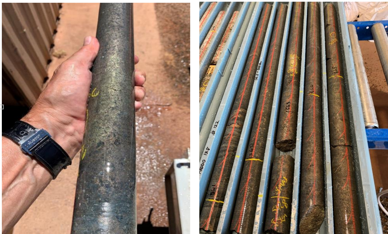
Image 1: Enriched copper sulphide interval (chalcopyrite - golden colour) hosted within a 6.2m-wide zone of massive and semi-massive nickel and copper sulphides in hole ANDD0128 at VC-07 West
