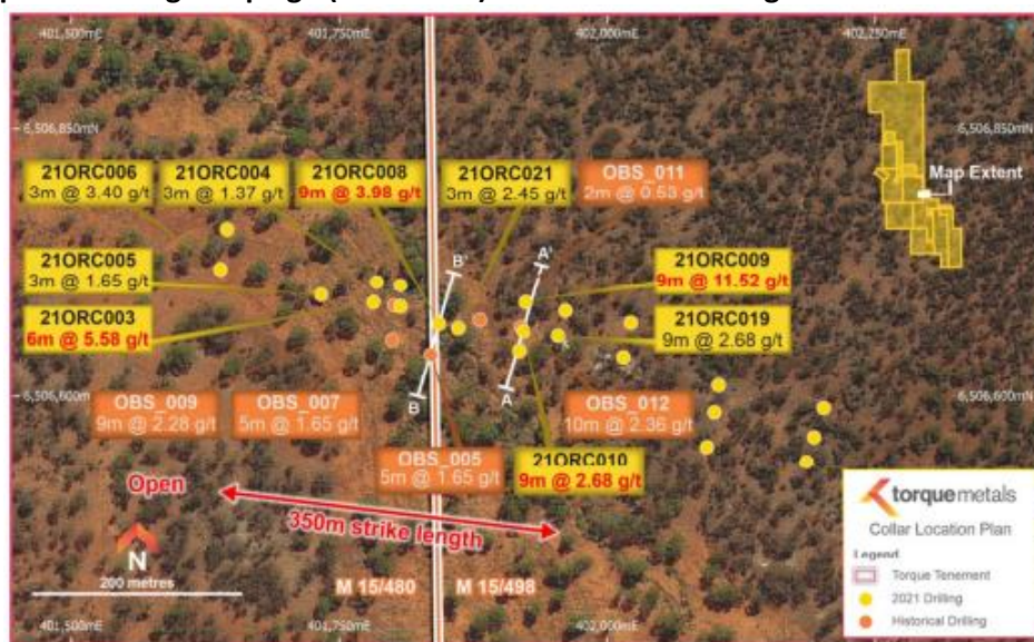
Figure 4: Collar location plan at Observation Prospect shows 350m strike length open to the West, East and at depth
