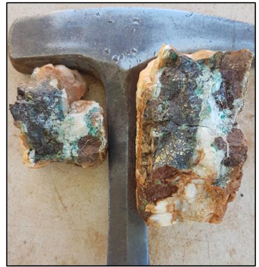
Figure 9: Rock chips samples of the high copper-gold vein at Tierra Prospect.
