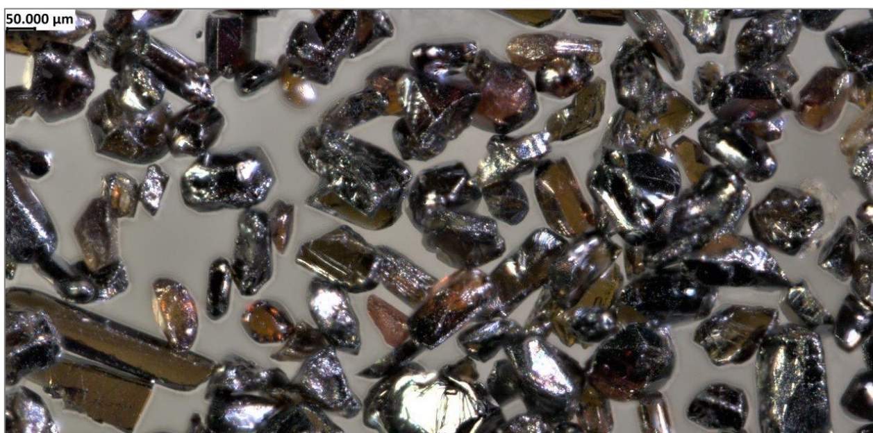
Figure 9: Photomicrograph of high purity rutile product 97.2% TiO 2 .
