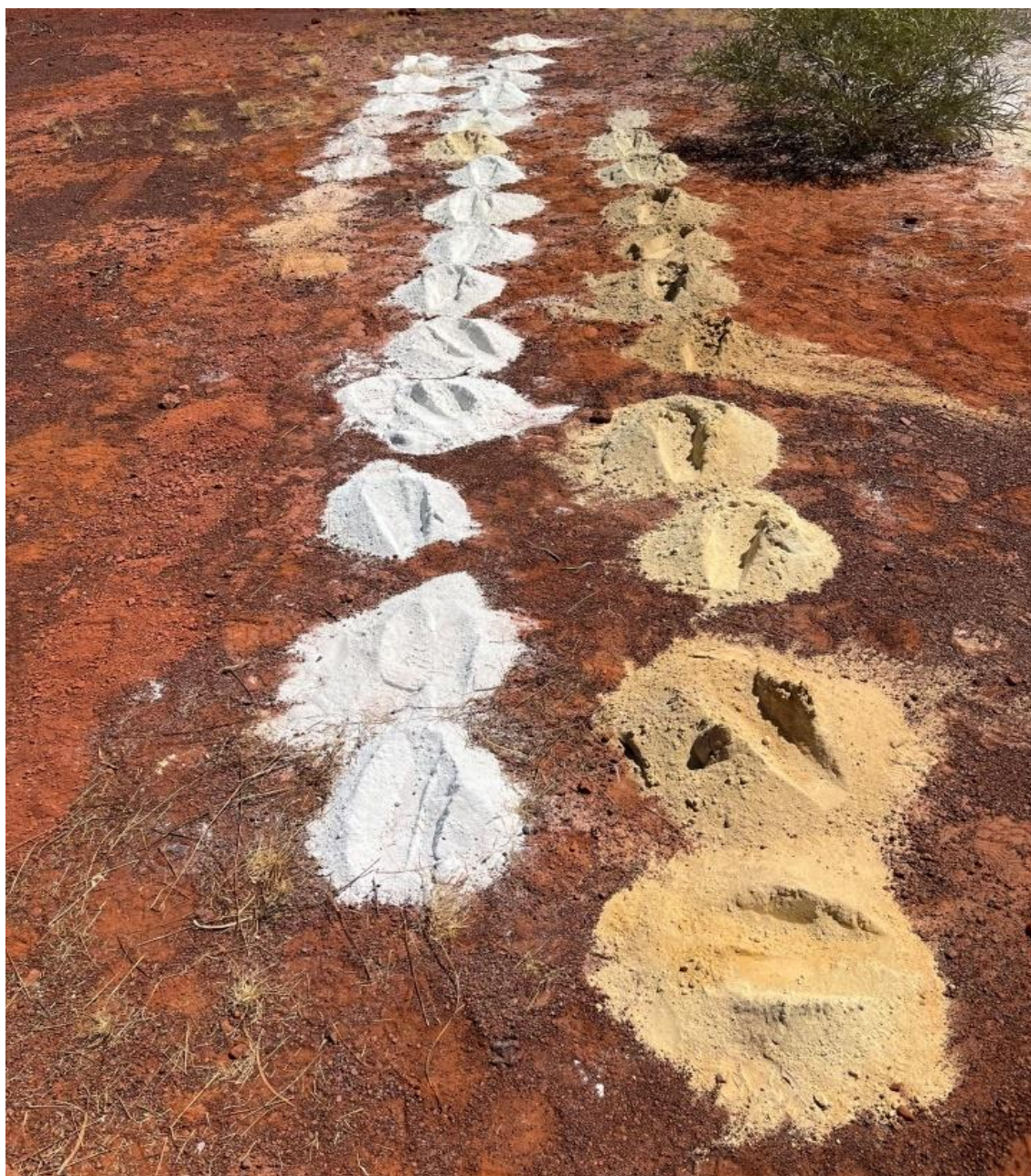
Figure 2 Photographs of typical drill soil from aircore holes drilled in the Tower area (21MAC021 and 21MAC029)
