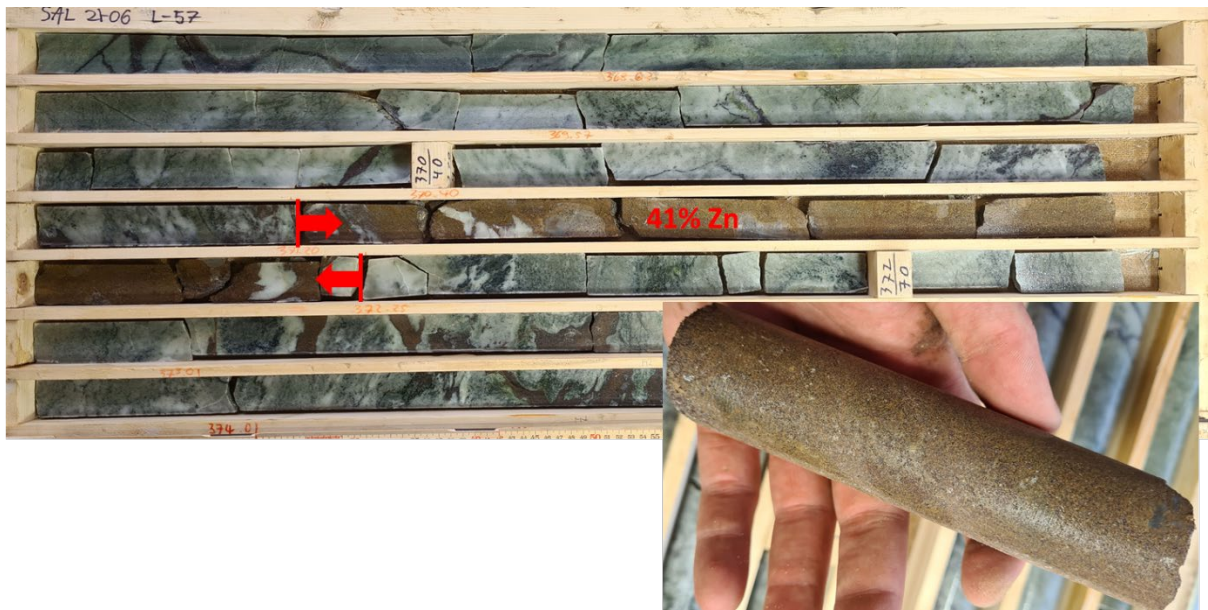
Figure 5: Half core from SAL2106 with 41% Zinc over 1.1m from 371.2m, part of larger interval of 14.0m @ 30 g/t Ag and 7.6% Zn from 365.5m. Inset image illustrating close up of the massive sulphide sphalerite mineralisation. (ASX 13/10/2021) 1
