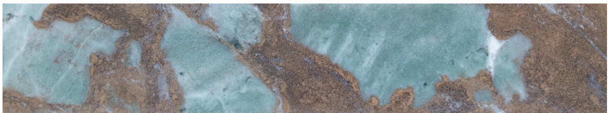
Figure 5a: Primary replacement sphalerite dominated mineralisation style at 410.8m in drill hole SAA08-003. All photos show core with 36mm in height. (ASX 13/10/2021) 1
