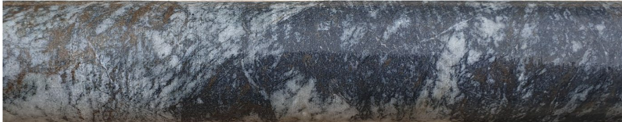
Figure 5e: Silver-rich, Galena dominated mineralisation style at 592.7m in drill hole SAL21-01. Interpreted to be partly remobilized mineralisation. (ASX 13/10/2021) 1
