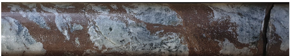
Figure 5c: Classic Sala style sphalerite breccia mineralisation style at 573.6m in drill hole SAL21-01. (ASX 13/10/2021) 1
