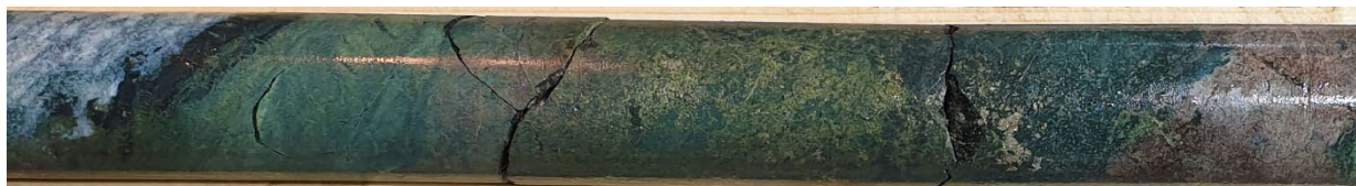
Photo 1: Drill core ST20-01 from 58.30m with visual sulphides of Chalcopyrite (visuals reported ASX:27/01/2021) (ASX: 20/04/2021 1 )
