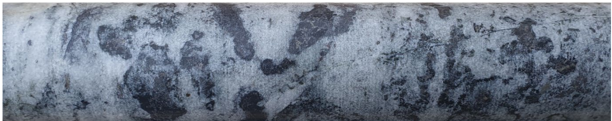
Figure 5b: Primary replacement galena dominated mineralisation style at 226.2m in drill hole SAL21-09 (ongoing). (ASX 13/10/2021) 1
