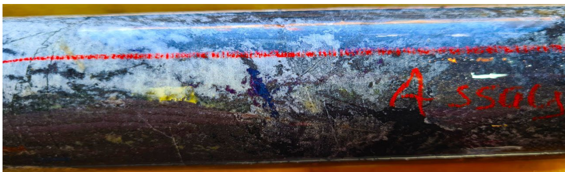
Photo 2: Drill core ST21-04 from 174.4m with visual sulphides of Chalcopyrite and Bornite (ASX: 20/04/2021 1 )
