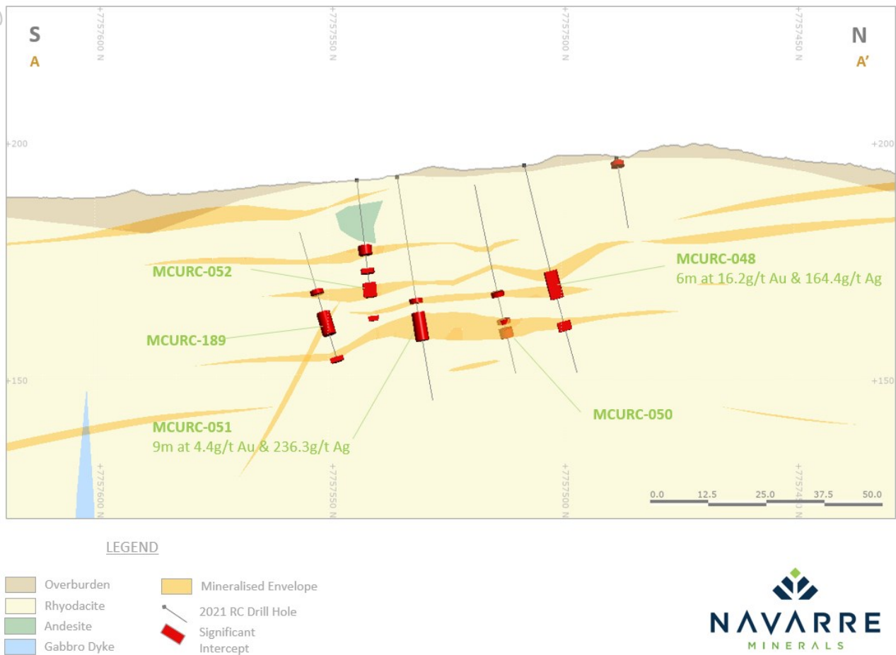
Figure 1: Schematic cross-section across Mount Carlton United
