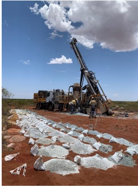
Photo 3: Strike Drilling T450 Aircore/Reverse Circulation Rig
