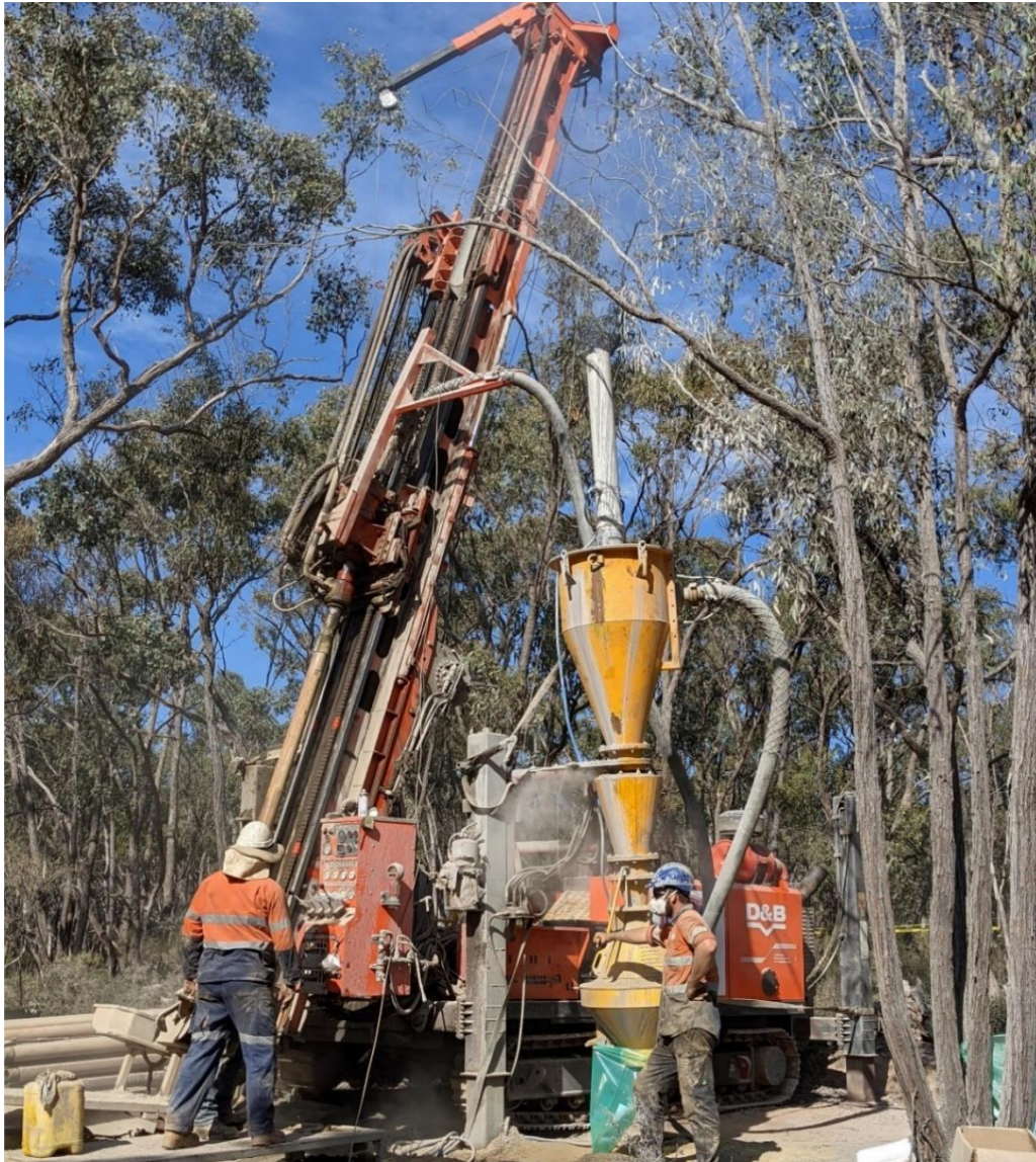
Figure 8: RC drilling at ~'s Reef prospect, South Muckleford Gold Project
