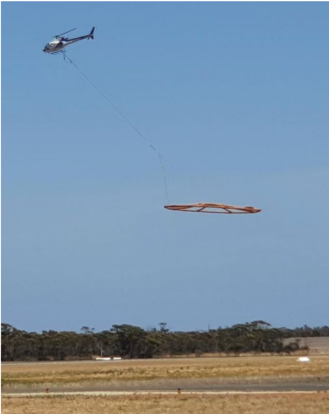
Figure 1 - Squirrel helicopter with NRG's Xcite electromagnetic system on site at Ravensthorpe (January 2022)
