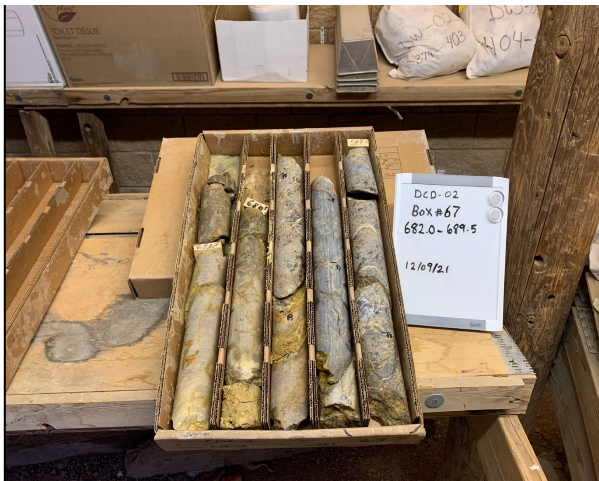
Figure 5: Drill core from hole DCD_02 at the Douglas Canyon Project showing silica matrix brecciated vein, and silica flooded host rocks
