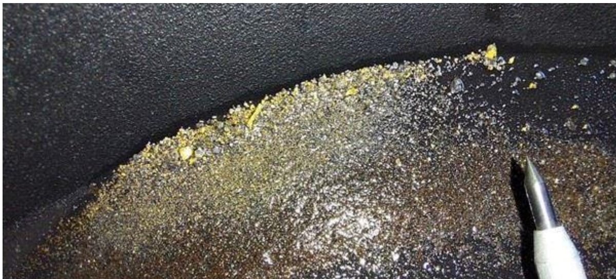
Photo 1: From a 360g sample split of drill hole 21MNRC007 : 70 to 71 metres, 1m @ 190.06 g/t (Photon 500g assay, MMG ASX Announcement 09 November 2021), panned concentrates displaying coarse gold and sulphides in the tails. The metal scribe tip shown is 8mm long, for approximate scale
