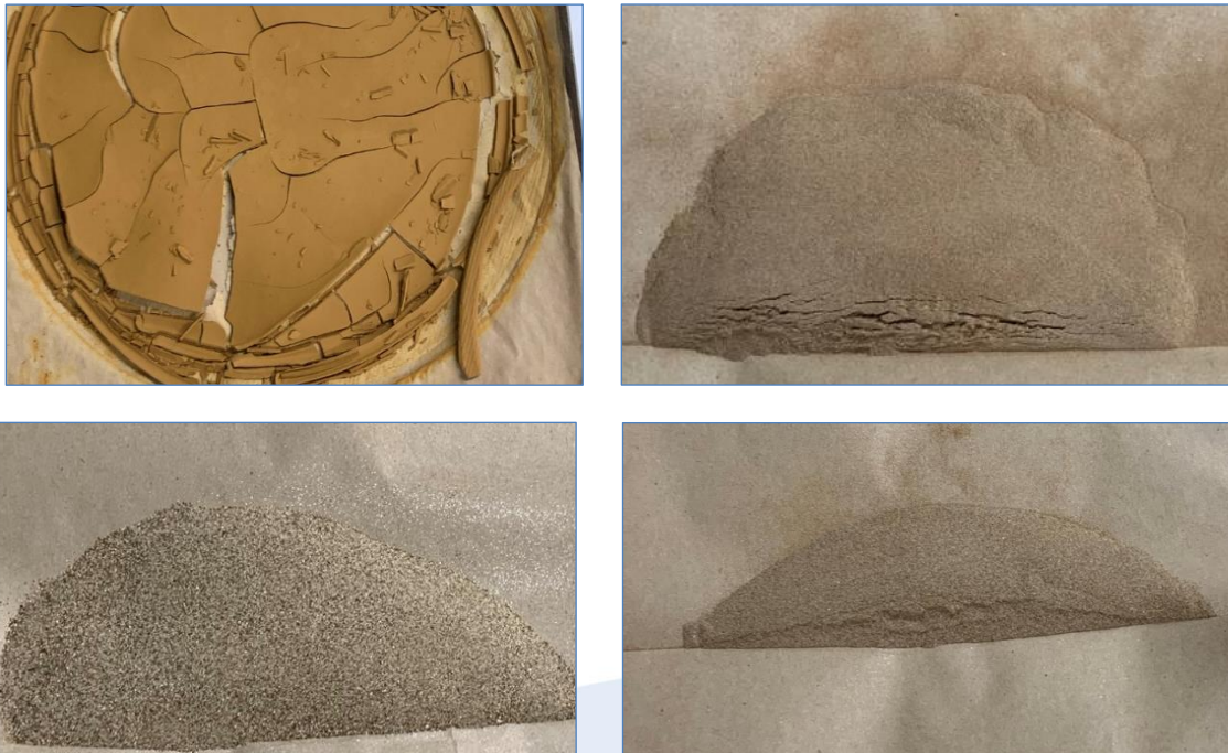
Figure 2: Sample fractions by size, clockwise from top left -20µm, +20µm -45µm, +45µm -75µm, and +75µm
