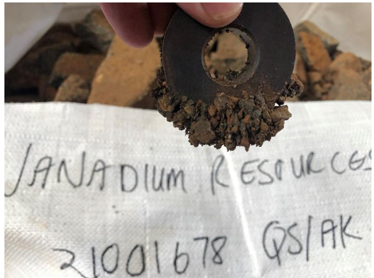
Figure 2 – Highly magnetic material contained in bulk samples
