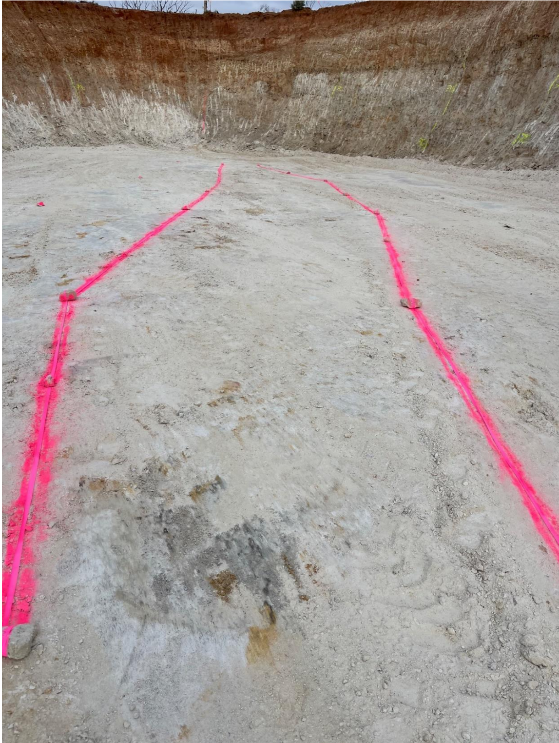
Figure 3: First ore mark-out on pit floor. Ore zone in-between pink lines.
