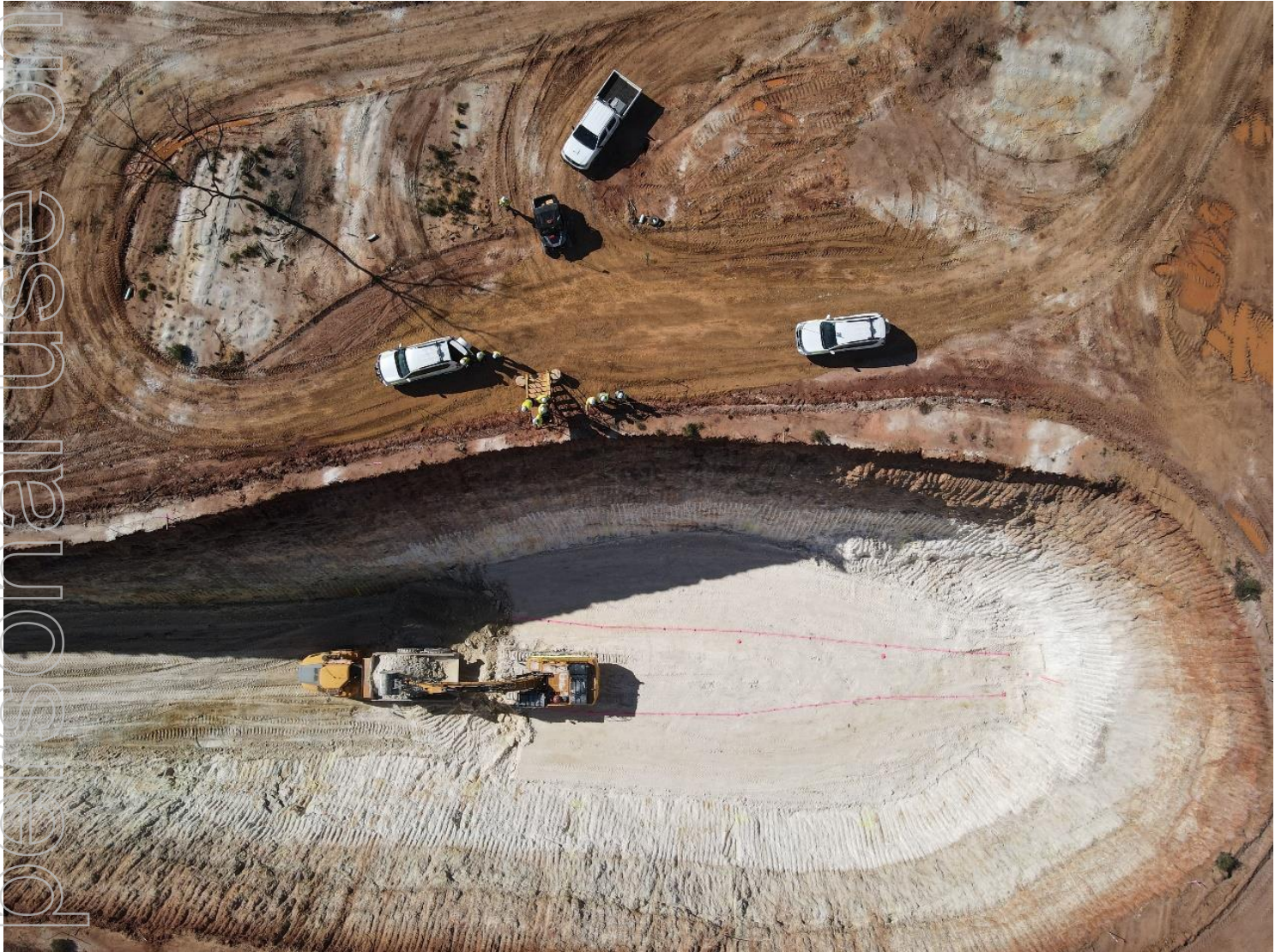
Figure 6: Aerial view of pit showing ore being mined in-between pink mark-out lines.
