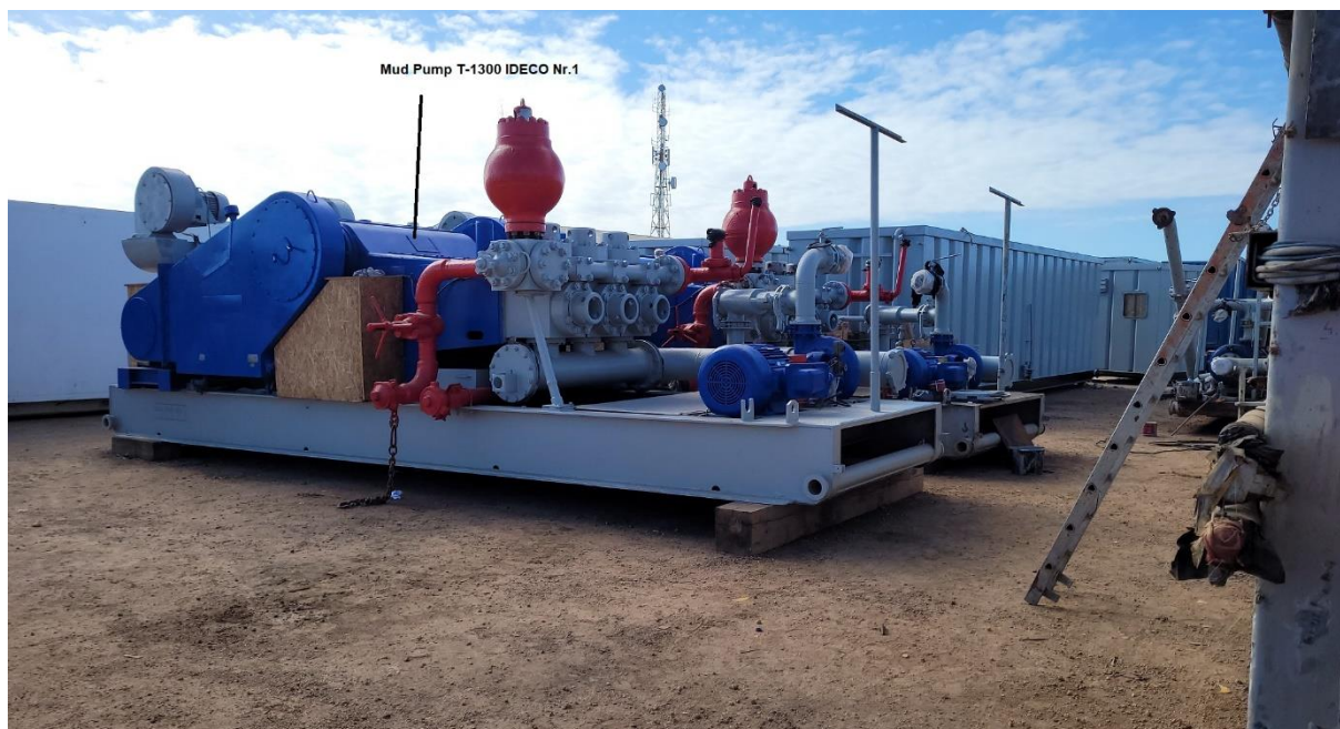
Figure 1 - Mud pump #1 T-1300 (47 tonnes) and Rig 202 equipment awaiting loading at Songo Songo Island jetty
