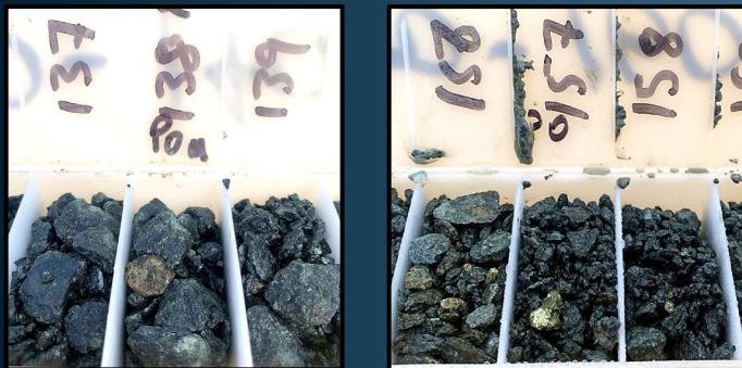
Example of disseminated sulphides in RC chips from the Callisto discovery (NRC268, downhole depths as marked. Logging records 1 to 5 % sulphide per one metre interval)
