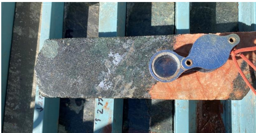
Photo 1: 21MHDD02- 282-283m (282.4m) - 1m @ 0.02% WO 3 , 0.23% Mo & 0.07% Cu - coarse grained visible molybdenite in magnetite skarn
