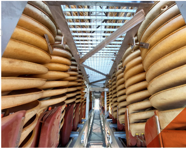
FIGURE 6: COBURN'S WCP SPIRAL FLOOR STRUCTURAL AND MECHANICAL CONSTRUCTION SUBSTANTIALLY COMPLETE
