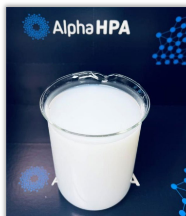
Sol-gel formation from high dispersible boehmite
