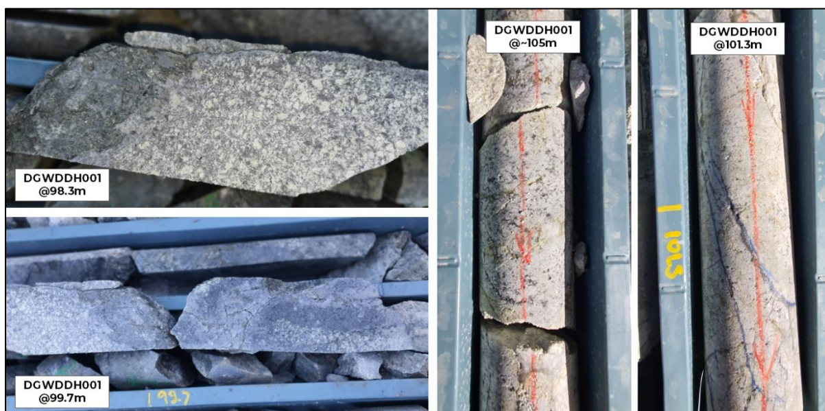
Figure 6: Porphyry intersected in DGWDDH001 from 88.9m to 110m displaying disseminated, fly-speck and veined chalcocite mineralisation
