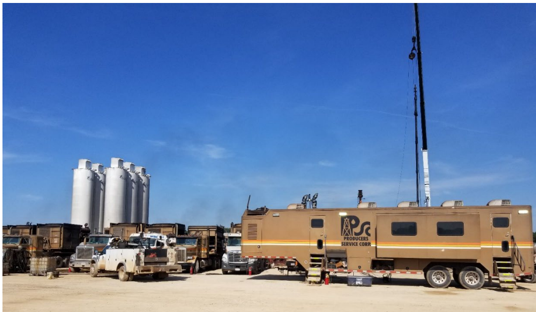
Figure 8. Producers Service Corp. (PSC) conducting multi-stage hydraulic stimulation operations on the Flames Well, Carter County, Oklahoma.
