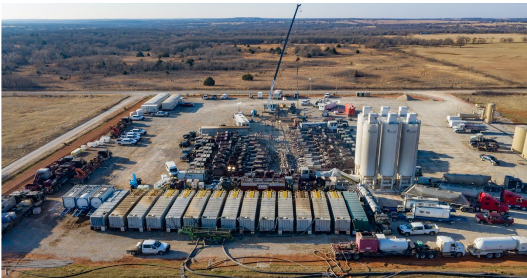
Figure 5. Rangers Well stimulation operations
